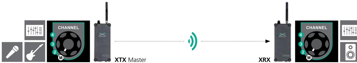
Transmitter XTX and receiver XRX are connected to each other within seconds – thus facilitating an easy introduction to the world of DIWA technology and providing the enjoyment of wireless audio transmission with high-level sound quality. The audio signal transmitted by the XTX can be received by an unlimited number of XRX receivers. Thus XIRIUM X becomes the preferred solution even with such a simple set up for numerous applications.
