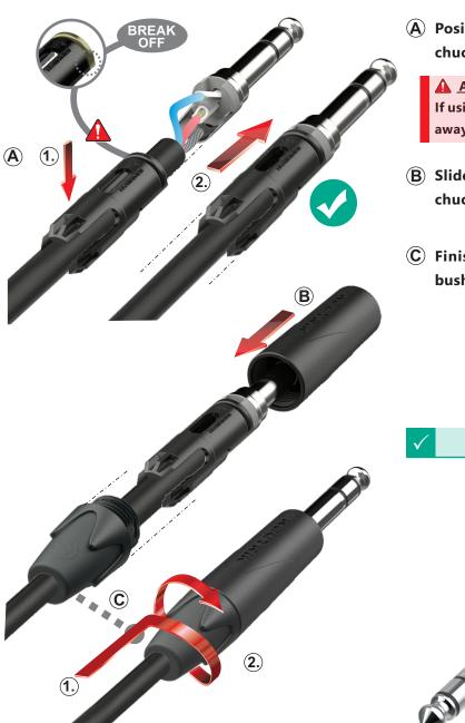
(A) Position the chuck onto the cable (1) and align chuck with plugfinger (2).
