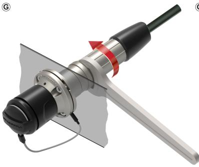
G Tighten the connector with the openend wrench.
