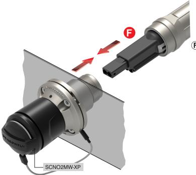
Position the connector housing into the front housing and tighten lightly.
