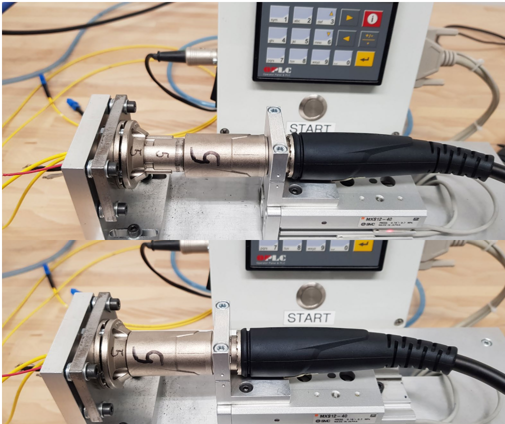
figure 6.b: fixture for 10.000 mating cycles
