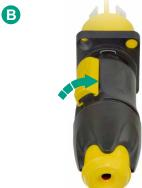
**Note:** After inserting properly as in illustration A, twist the cable connector clockwise to lock.
