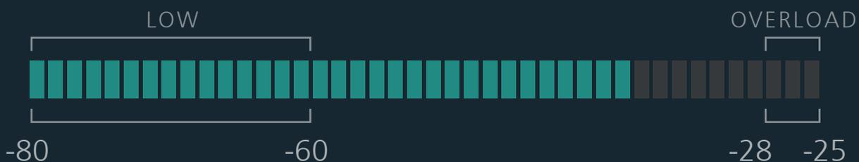
Good signal quality is not only measured by having the highest RSSI level. It's more important to have low packet loss (i.e. green bars). When necessary, engage the RX -30 dB attenuator in the app by setting it to ON.
