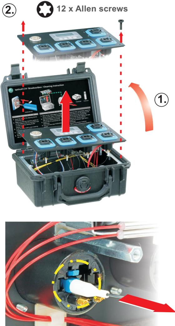
1. Open the breakout box and clean the surface with a lint free wipe FOCD-DW
