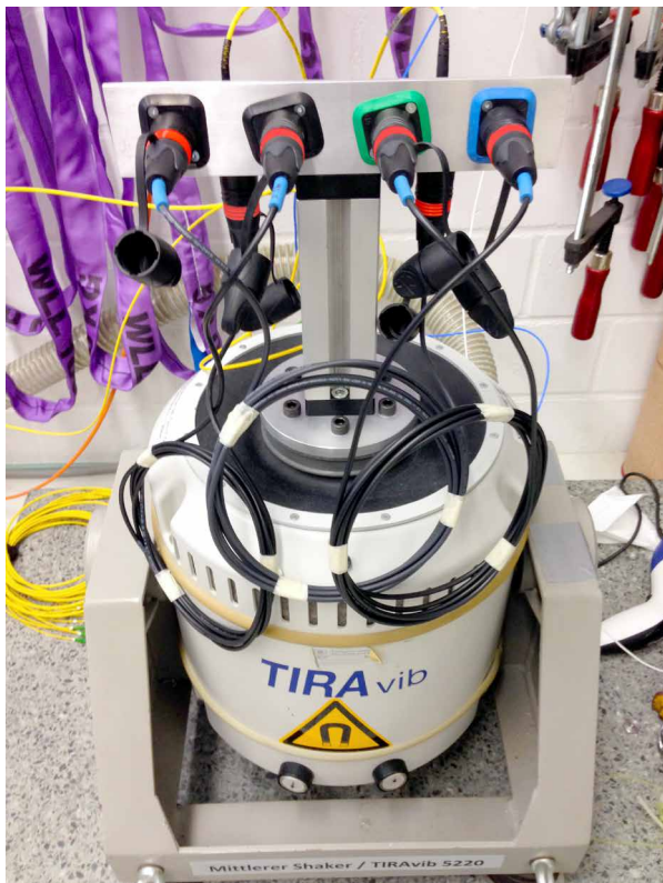
figure 2.a: : Vibration equipment and test cable arrangement
