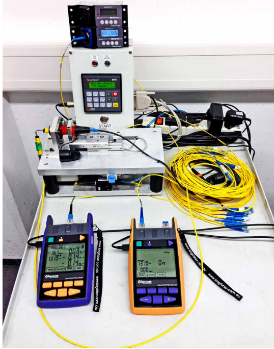
figure 6.a: measuring setup for durability and lifetime test
