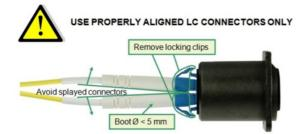
Avoid splayed connectors by using LCs without anti-snag collars and a boot diameter < 5 mm (available from suppliers as e.g. Corning).
